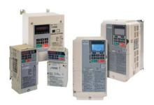
Many automation products are now equipped with built in preventative maintenance tools. Variable frequency drives are designed with *life monitors* that proactively provide the maintenance team with information that will help avoid downtime. The drive sends out notifications and warnings when consumable components like cooling fans, DC bus capacitors, inrush relays, and IGBTs are nearing the end of their predicted lifespan so that they can be replaced prior to failure during operation.
